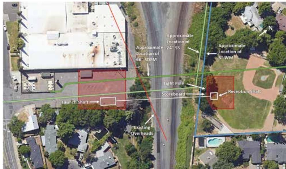
Figure 1. Aerial view of guided boring crossing of the two sets UPRR tracks showing key project constraints. Work areas are shown shaded in red.
